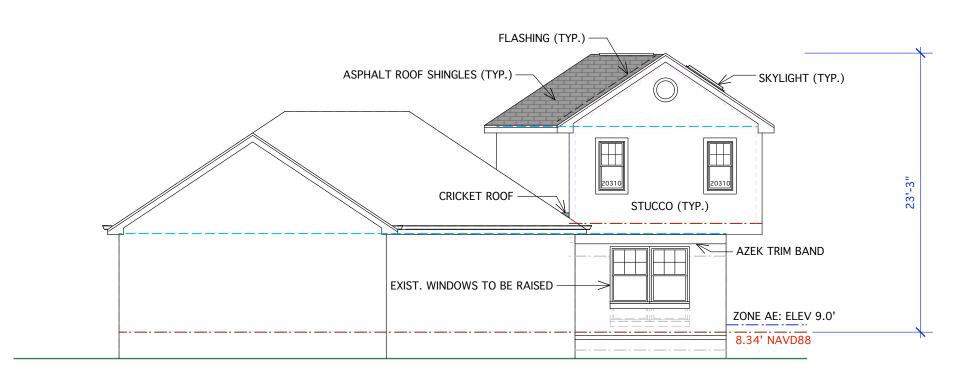
PARTIAL FRONT ELEVATION SCALE: 1/8" = 1'
