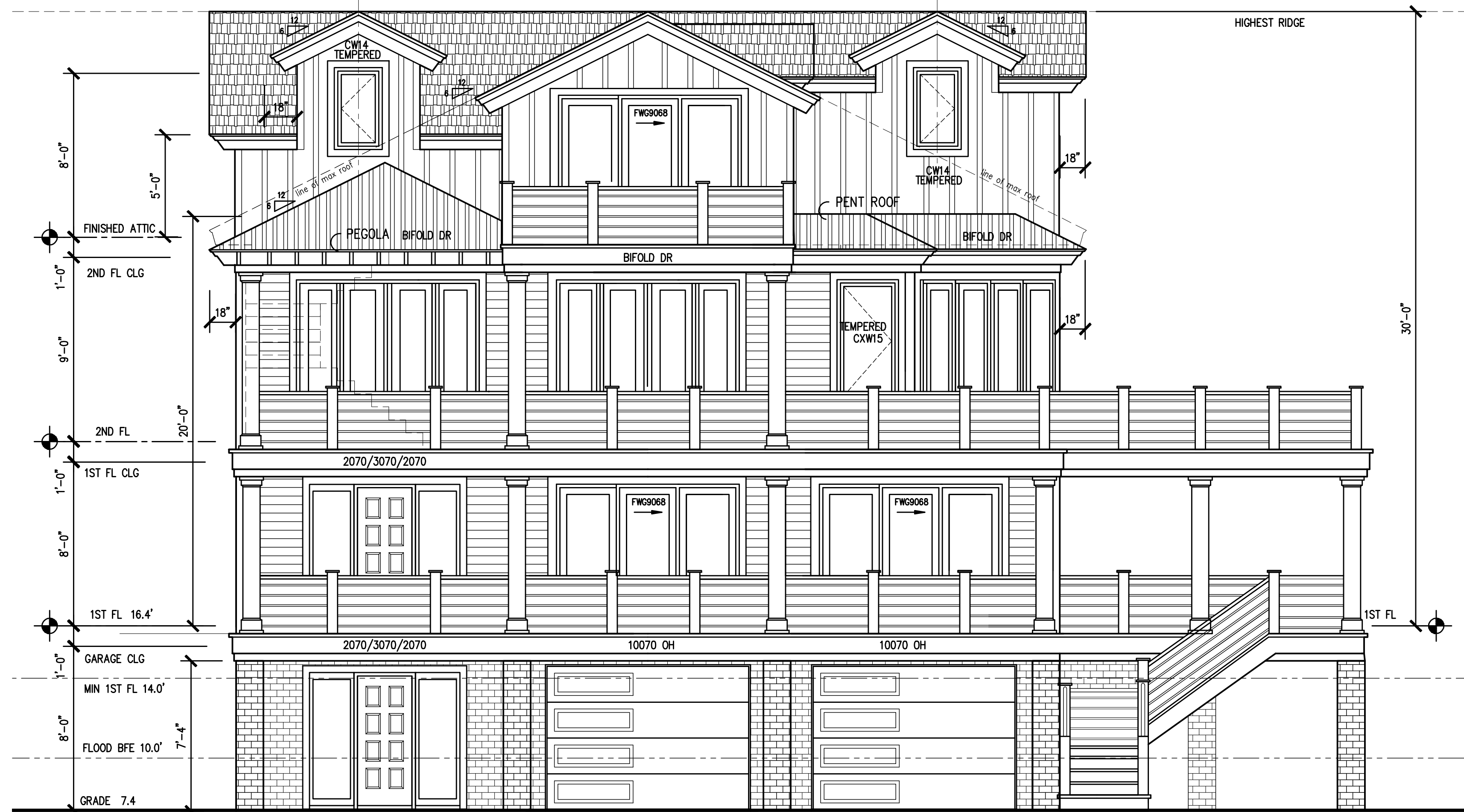
FRONT ELEVATION SCALE: 1/4"=1'-0"
